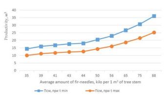
Figure 4: Dependence of the output per shift of the mobile unit on the average number of fir-needles kg, per 1 m<sup>3</sup> of tree stem under favorable and unfavorable conditions
