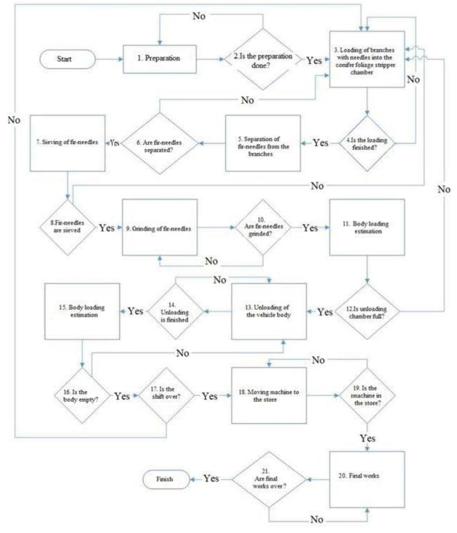
Figure 2: Information-logical model of the mobile unit process
